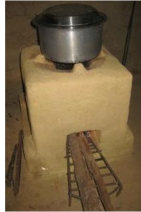
Figure 2: A typical mud ICS replaced
